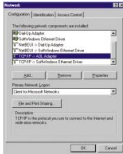
Fig 3 Remove the TCP/IP protocol and Winsock files if you think they've been overwritten by software such as AOL
